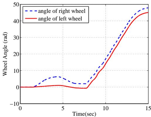
Fig. 18. Wheel Angles as the One Hand Propulsion Control Result
