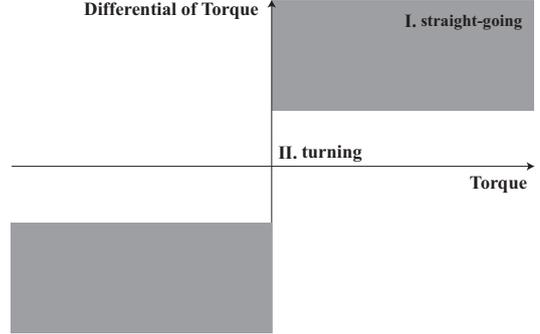
Fig. 16. Division of the Torque Phase Plane for One Hand Propulsion
