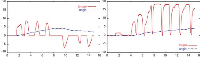
Fig. 3. Necessary Torques to Drive a Wheelchair (Upper: drive on level ground, Lower: drive on hill)
