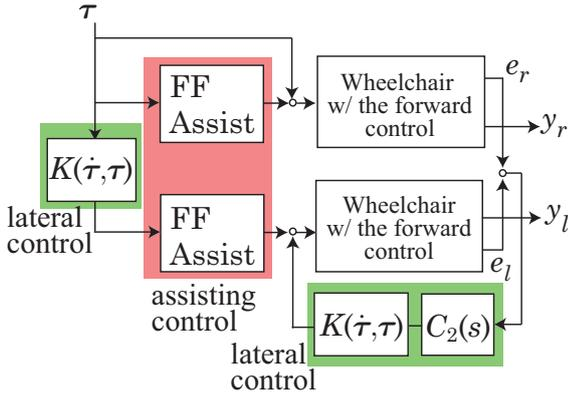
Fig. 14. Controller with the Synchronization Function  $K(\dot{\tau}, \tau)$
