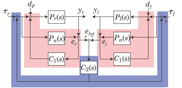
Fig. 6. Structure of Lateral Disturbance Rejection Controller - Force Control Type
