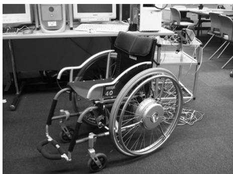
Fig. 1. Commercial Power Assisting Wheelchair
