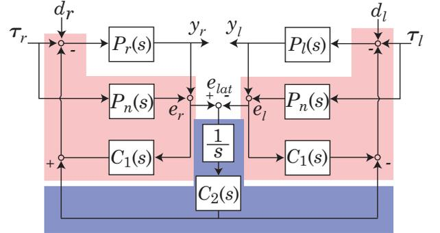
Fig. 7. Structure of Lateral Disturbance Rejection Controller - Position Control Type
