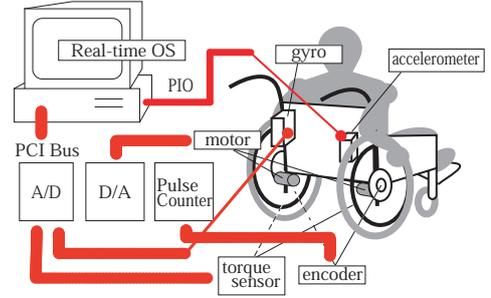
Fig. 8. Modified Assisting Wheelchair
