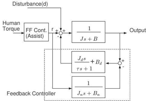
Fig. 4. Structure of Forward Disturbance Attenuation Controller
