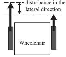
Fig. 5. Definition of Lateral Disturbance
