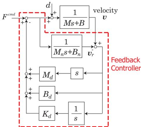
Fig. 5. Impedance Control by Velocity Feedback Control
