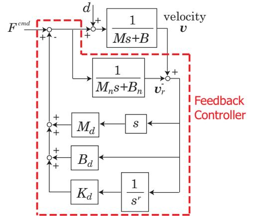
Fig. 6. Structure of Fractional Impedance Control
