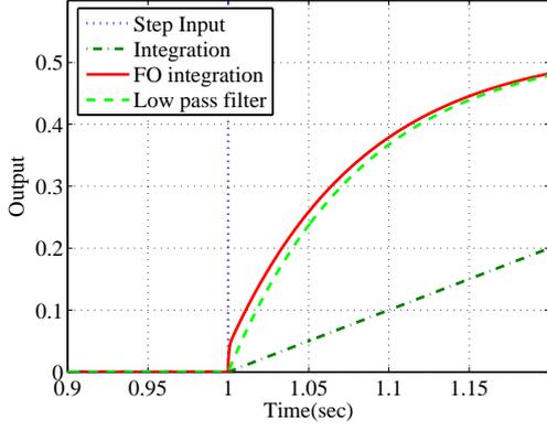
Fig. 7. Step Response of Approximated Fractional Order Integrator
