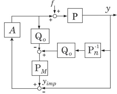
Fig. 9. Blocks of Force-sensor-less Power Assist Control
