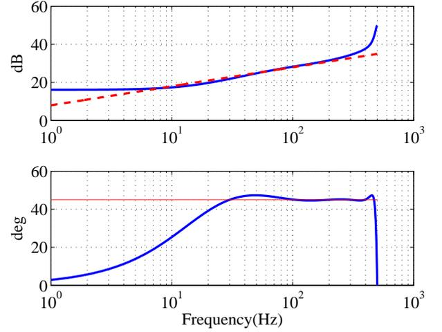
Fig. 3.  $s^{0.5}$  Discretized by the CFE Approximation
