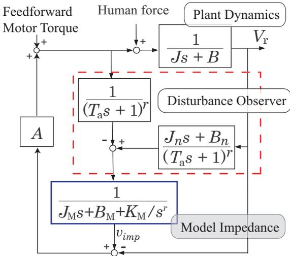
Fig. 8. Force-sensor-less Power Assist Control Incorporating Fractional Order Calculus
