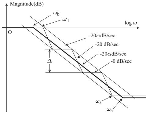
Fig. 1. An Example of Broken-line Approximation (N = 3)
