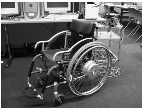
Fig. 1. power assisting Wheelchair as an Example of Power Assistance Tools (YAMAHA JW II)
