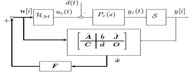
Fig. 3: Multirate control with disturbance observer.
