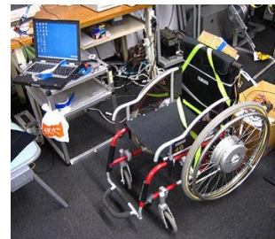
図1 Power-assisted wheelchair as an experimental tool (YAMAHA JW II)
