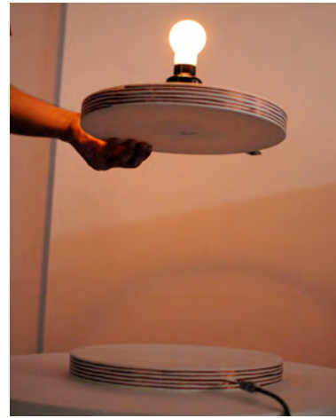
Fig. 11. Experiment of Wireless Power Transfer at Hori Lab.
