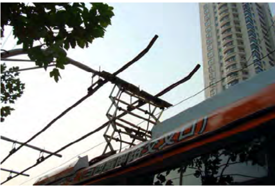
Fig. 5. Illustration of Charging an EV at a Bus-stop (Charging Duration: less than 30 s).
