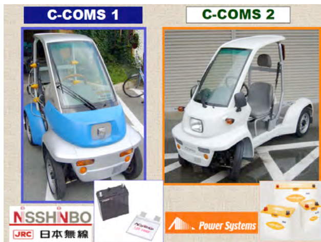
Fig. 2. C-COMS Driven Only by Supercapacitors.
