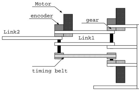
Fig.3 Outline view of robot arm design
