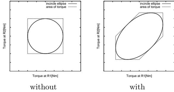
Fig.2 Range of Joint Torques with or without Bi-articular Muscles
