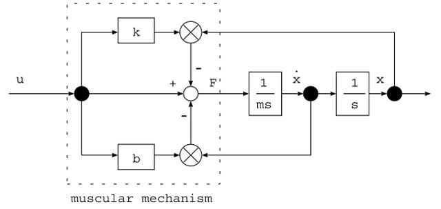
Fig. 8. Block diagram to realize muscular viscoelasticity
