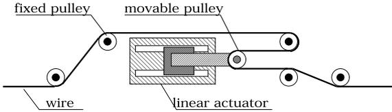
Fig. 7. Bi-articular driving mechanism using pulleys
