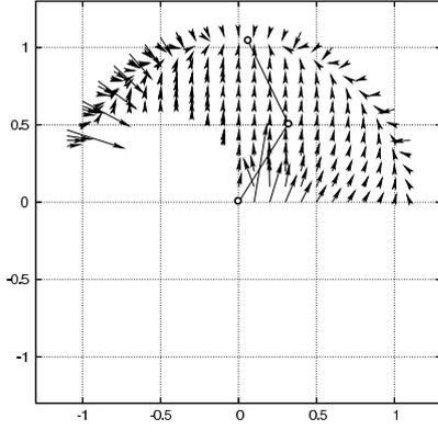
Fig. 4. Output force at end point when arm deflects from equilibrium position
