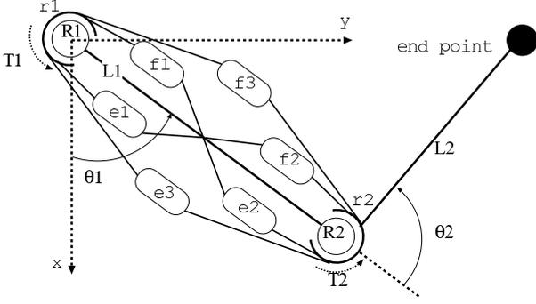
Fig. 2. Two joint link model with both mono-articular muscles and bi-articular muscles
