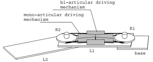
Fig. 9. A complete implementation of the animal arm model shown in Fig. 2
