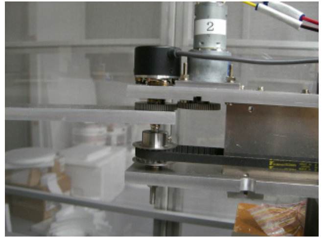
Fig. 10. Detail of actual bi-articular driving mechanism (R2 side)
