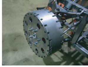
Fig. 3 In-wheel motor
