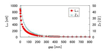
Fig.13. Optimized parameters of mutual inductance and characteristic impedance with maximum efficiency at each air gap length.
