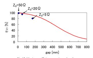
Fig.12. Maximum efficiency vs. air gap length. The line is the theoretical result, and the dots are the results of experiments.
