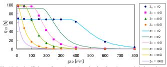
Fig.10. Peak efficiency for each gap length related to characteristic impedance. Dots denote the results of electromagnetic field analysis, and lines denote the theoretical results based on equivalent circuits.
