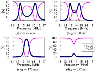
Fig.4. Results of electromagnetic field analysis for efficiency vs. frequency at different gap lengths.
