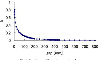
Fig.6. Coupling coefficient k vs. gap length.
