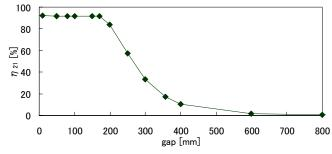
Fig.5. Results of electromagnetic field analysis for peak efficiency vs. air gap length.
