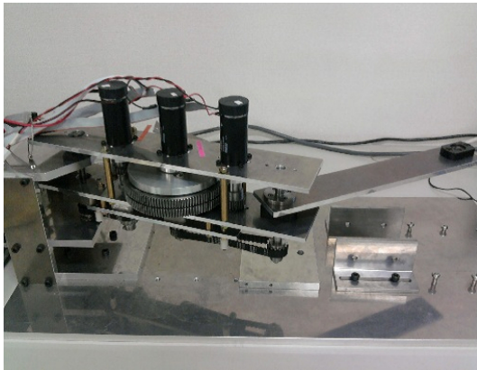
Fig. 16. Two-link Robot Arm With Biarticular Driving System
