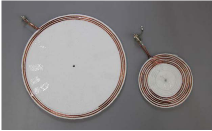
Figure 1. Antennas(left: \phi 300mm antenna, right: \phi 150mm antenna).
