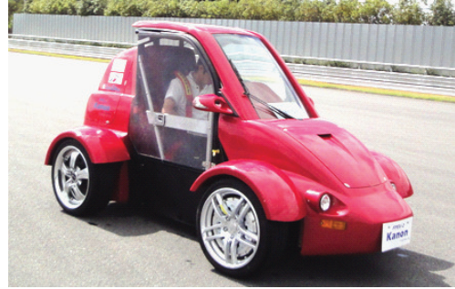
Figure 6: Experimental in-wheel-motor-driven electric vehicle.
