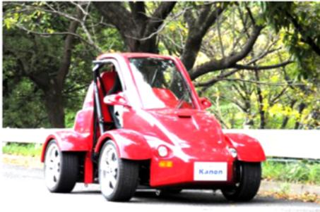
Figure 12. In-wheel-motor-driven electric vehicle.
