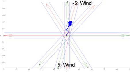
Fig. 10. Effect of a lateral wind force (simulation with noise) of 300N in the feature space. It is not detected as a failure in the lateral acceleration sensor.
