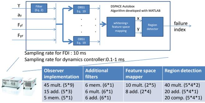
Fig. 13. Overview of the RT implementation of the obs. based FDI scheme
