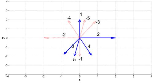
Fig. 6. Fault directions in the feature space  $(x, y)$  (1:  $f_{s1} = \Delta a_y$ , 2:  $f_{s2} = \Delta \gamma^*$ , 3:  $\Delta u_1 = \Delta F_{yf}$ , 4:  $\Delta u_2 = \Delta F_{yr}$ , 5:  $F_w$ )
