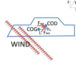
Fig. 3. Modelling of cross wind influence on the vehicle
