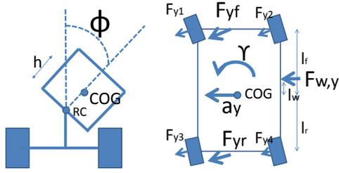
Fig. 2. Kinetic relationships for vehicle modelling, ( $\gamma$ : yaw rate,  $F_{yf}, F_{yr}$ : front, rear lateral force,  $a_y$ : lateral acceleration,  $F_{w,y}$ : crosswind force,  $\phi$ : roll angle)
