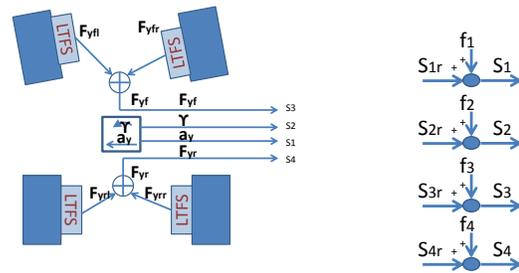
Fig. 1. Left: Sensor concept for lateral vehicle dynamics for EVs with LTFS Right: Additive sensor fault model
