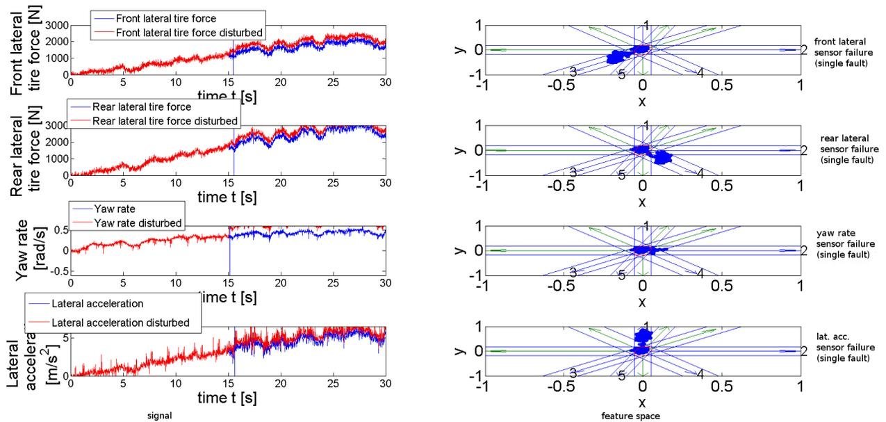
Fig. 9. Experimental results with artificially added single sensor failures (drift), their representation (right) in the feature space (Faults occurring at  $t = 15s$ , blue vertical line shows time instant, when error is detected). The left diagrams show the disturbed signals (red) together with the correct signals (blue).
