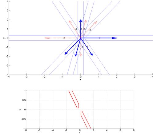
Fig. 7. Top: Regions where an unambiguous single fault detection is possible (within two blue lines, where there is no intersection with other "strips") Bottom: Exemplary the region in the feature space for unambiguous rear lateral tire force sensor fault detection is shown.
