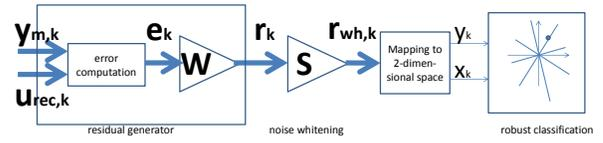
Fig. 5. Fault detection and isolation scheme (residual generator realized with residual observers)
