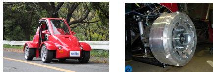
Fig. 1. Experimental vehicle (left) and in-wheel motor (right).
