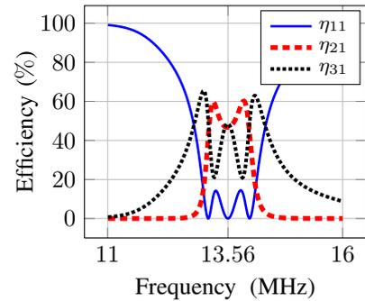
Figure 9. Simulation result of equal power distribution considering internal resistance after impedance matching.
