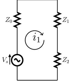
Figure 4. Simplified two-receiver circuit.
