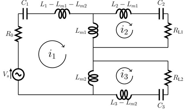
Figure 3. Alternative circuit of two-receiver wireless power transfer.
