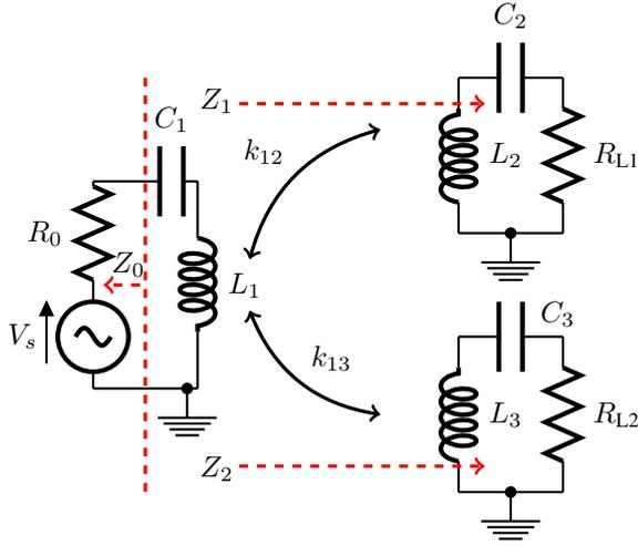
Figure 1. Equivalent circuit of a two-receiver system.
