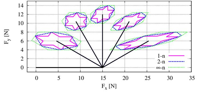
Fig. 4. Comparison of maximum output force at end effector —  $\theta_2 = (30, 60, 90, 120, 150^\circ)$
