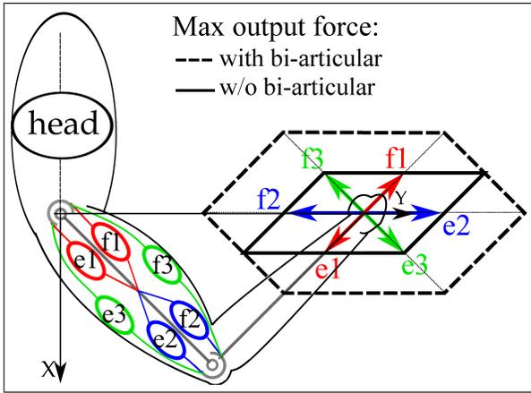
Fig. 1. Two-link arm with four mono- and two bi-articular muscles: model and resulting forces at the end effector
