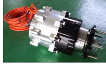
(b) In-wheel motor
