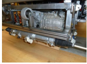
(a) OBM with differential gear
