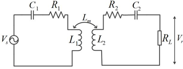
Fig. 2. WPT equivalent circuit
