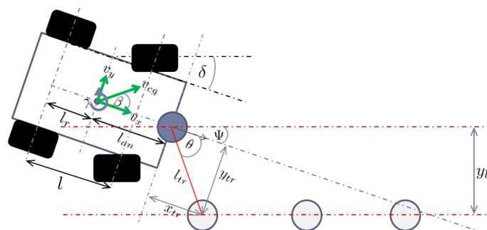
Fig. 1. Schematic of electric vehicle with WPT receiver
