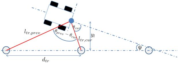
Fig. 5. Vehicle with wireless power transmitter alignment
