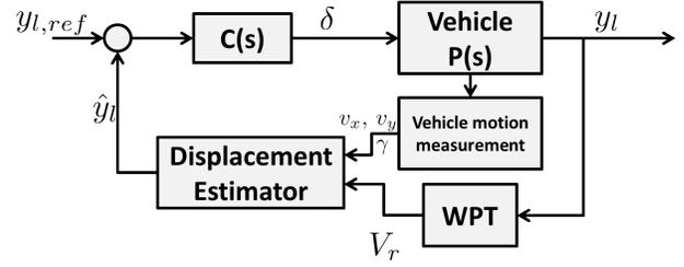
Fig. 8. Control system block diagram
