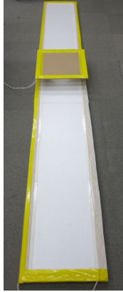
Figure 3. Fabricated 3 meter coil and receiver coil
