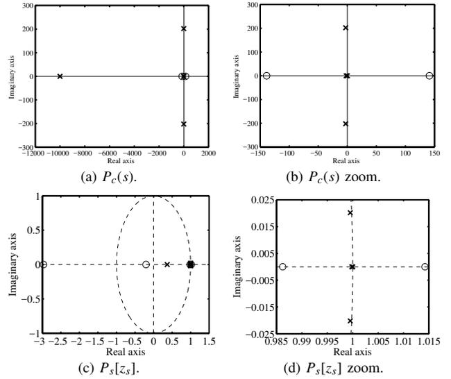
Fig. 7. Pole-zero map of  $P_c(s)$  and  $P_s[z_s]$ .
