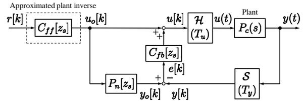
Fig. 8. Approximated plant inverse feedforward control configuration. Simulation block diagram for NPZI, ZMETC, ZPETC methods.
