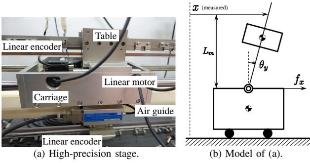
Fig. 5. Experimental high-precision stage and its model for simulation[24], [6], [30].
