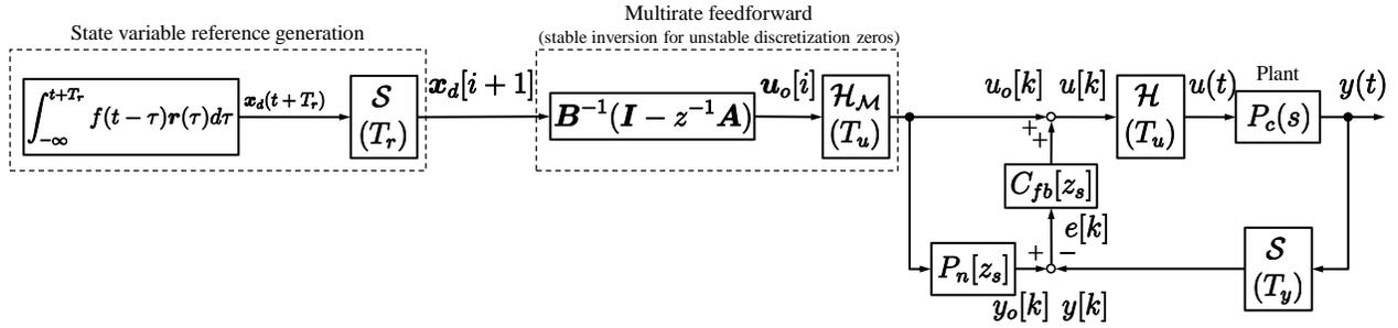
Fig. 3. Perfect Tracking Control method based on multirate feedforward proposed in reference [22].  $S$ ,  $\mathcal{H}$ ,  $\mathcal{H}_M$  denote a sampler, a holder, and a multirate holder, respectively.  $z$  and  $z_s$  denote  $e^{sT_r}$  and  $e^{sT_u}$ , respectively.
