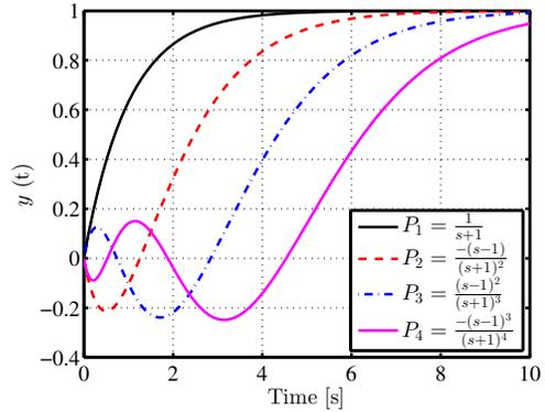
Fig. 1. Step response comparison.  $P_1$  is 1st order transfer function without unstable zero.  $P_2, P_3, P_4$  have one, two, three unstable zero(s) as shown in the legend of the figure. Step responses of the system with unstable zero(s) make undershoot.
