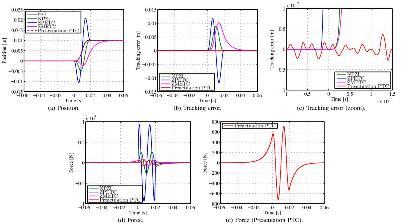
Fig. 10. Simulation results of the plant with continuous time unstable zero. From (c), the perfect tracking is achieved for every  $T_r = 500 \mu\text{s}$ .
