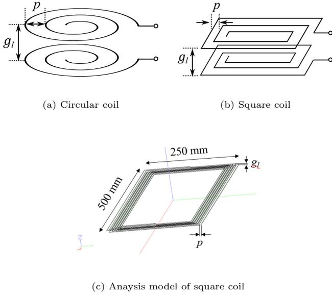
Fig. 4 Double layered open end spiral coil
