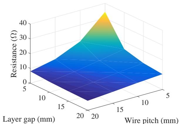
Fig. 11 AC resistance vs. coil parameter plot
