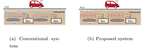
Fig. 3 Diagram of conventional and proposed system
