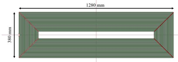
Fig. 6 Designed simulation model of 85 kHz self-resonant coil
