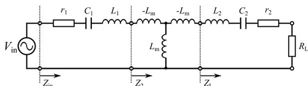
Fig. 1 Equivalent circuit of S/S type wireless power transfer system
