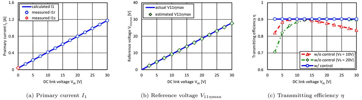
Fig. 6 Simulation results of reference voltage calculation and efficiency maximization.
