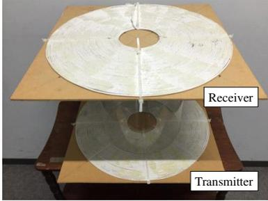
(b) Transmitter and receiver coils.
