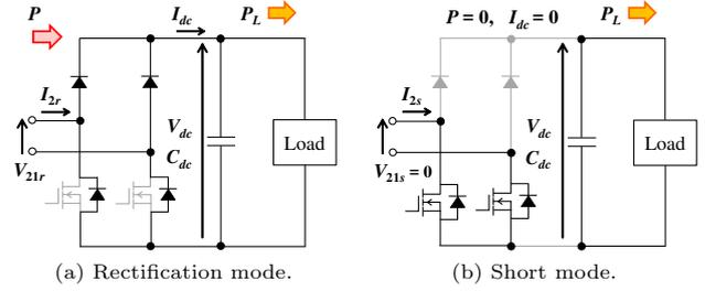
Fig. 3 Operation modes of Half Active Rectifier.
