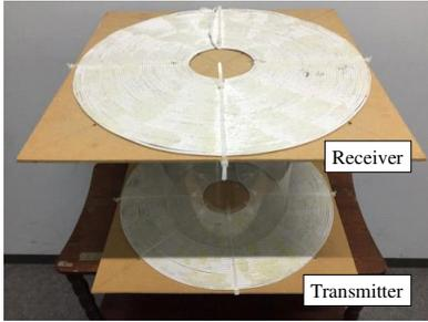
(b) Transmitter and receiver coils.
