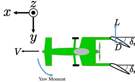
Fig. 8. Relation between rudder and yaw moment.
