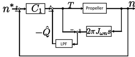
Fig. 9. Block diagram of propeller's revolution controller.
