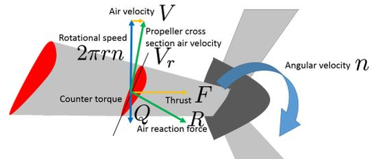
Fig. 5. Physics of propeller.
