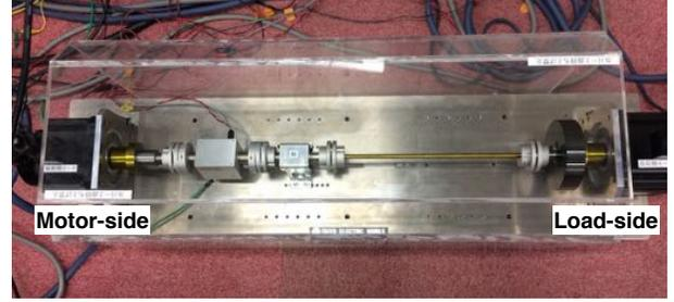
Fig. 5: Experimental machine of two-mass motor bench
